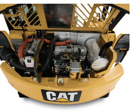
Robust, reliable and easily serviceable are the key attributes of Cat® Mini Hydraulic Excavators. Full steel body work panels and protected front linkage lines are routed neatly out of the way of potential damage above the boom. Easy access to all daily service points are accessed through the rear hood and side cover. A 500 hour engine oil change period lowers operating costs and the Cat S•O•S<sup>SM</sup> points assist easy oil sampling for preventative maintenance checks.
