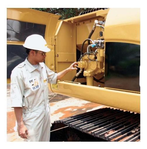
**Ground Level Service.** The design and layout of the 320D was made with the service technician in mind. Many service locations are easily accessible at ground level allowing critical maintenance to get done quickly and efficiently.
