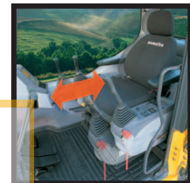
Seat Sliding Amount: 340 mm 13.4", increased 120 mm 4.7"
